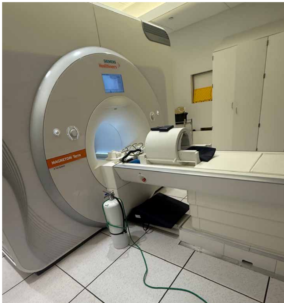
FIGURE 2. Testing the 9L Water Mist Fire Extinguisher during exposure to a 7-Tesla MR system. Note the lack of magnetic field translational attraction for this product while in front of the opening of the bore of the 7-Tesla MR system (i.e., a worst-case position in relation to the 7-Tesla MR system), as evidenced by the slack in the rope that was attached to this device.
